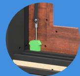
Dual top and bottom pins engage and disengage the hinging feature. The cartridge System guides the pin smoothly.
