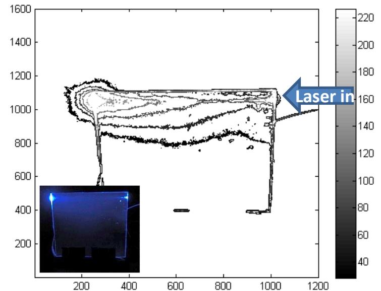
Here is reported the blue light outcome in a panel without scattering particles (up right) with respect to a panel with scattering particles (down right).
